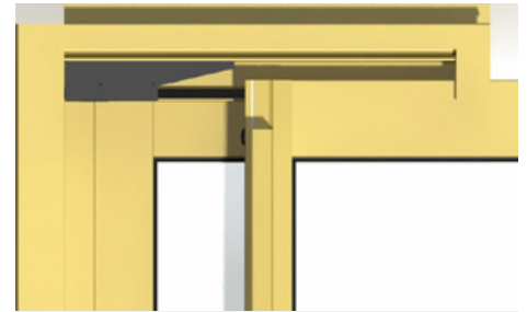
Tapered sash buffer stop to keep panel on the track.
